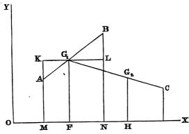
the plane of the paper,  $P_1$ ,  $P_2$ ,  $P_3$  ...,  $P_n$  their weights, and OX, OY two fixed straight lines intersecting at right angles in O.
